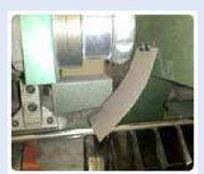
Too much drag with the springs will cause the signature to pop forward. The good news is you can bend and shape the spring as needed. Need more pressure? Double up on the spring or add a piece of steel strapping or similar material.
