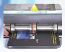
There are several factors which affect the quality and performance of a crease. These include the rule width (male component), the depth of crease, the width of the female channel, and the 'critical distance' (the distance from the side of the male rule to the edge of the female channel.)
